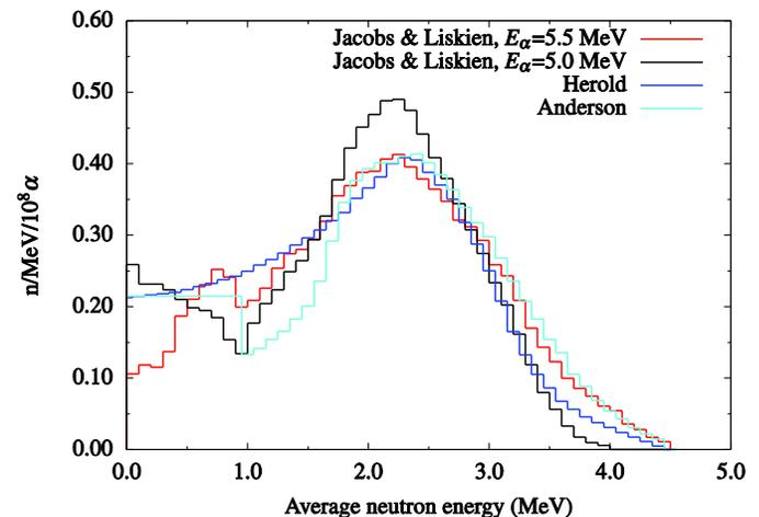
Fig. 9. Neutron energy spectra from SOURCES 4C calculations and measurements of Jacobs and Liskien, Herold, and Anderson.
