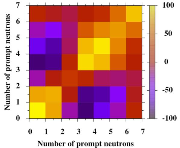
Fig. 9. Correlation matrix (%) for the  $^{240}\text{Pu}$  spontaneous fission neutron multiplicity based on results of the FREYA calculations.
