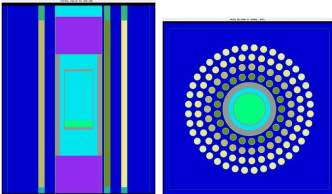
Fig. 8. Vertical and horizontal cross section views of the ENMC geometry, showing the central measurement cavity and  $\text{PuO}_2$  material (1) and 121  $^3\text{He}$  tubes in four rings (2).
