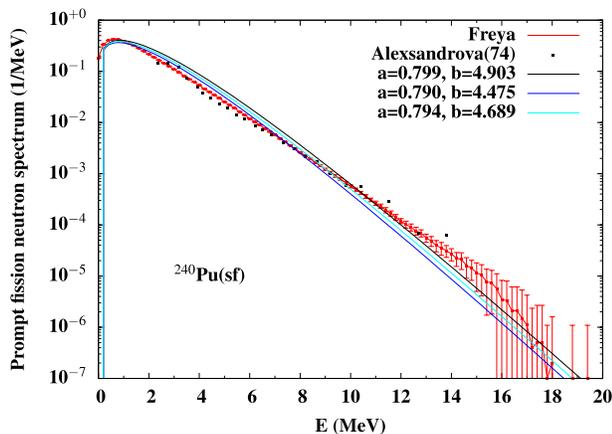
Fig. 8. FREYA-generated neutron energy spectrum for  $^{240}\text{Pu}$  spontaneous fission based on the excitation energy parameter,  $\chi$ , uncertainty of Schillebeek [30]. Also shown is the default Watt fission spectrum based on spectrum parameters used in MCNP. [Note: remove the Watts spectrum uncertainty lines]
