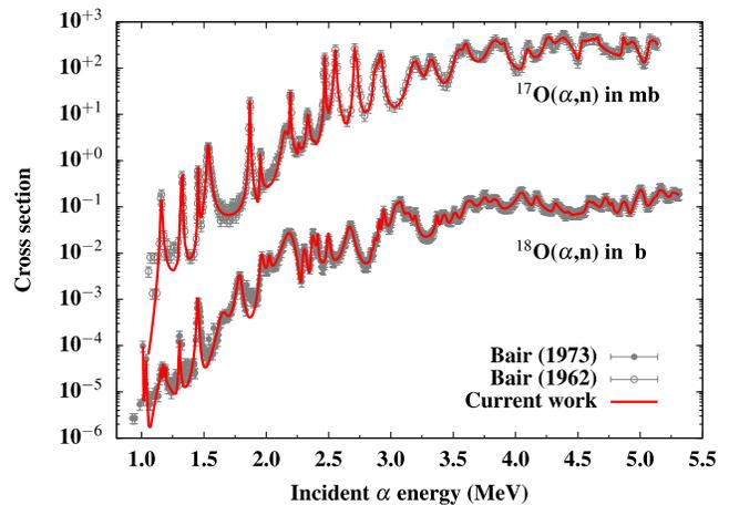
Fig. 2. Bair's experimental data for  $^{17,18}\text{O}(\alpha,n)$  cross sections and the cross section evaluations performed in this work using the SAMMY code.
