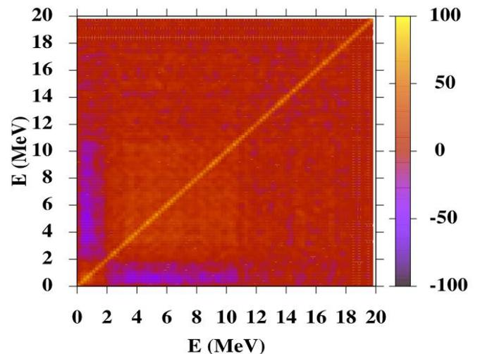
Fig. 10. Correlation matrix (%) for the  $^{240}\text{Pu}$  spontaneous fission neutron energy spectrum based on results of the FREYA calculations.
