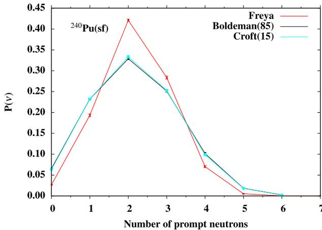
Fig. 7. FREYA-generated neutron multiplicity for  $^{240}\text{Pu}$  spontaneous fission based on the excitation energy parameter,  $\chi$ , uncertainty of Schillebeek [30] compared to other evaluations.
